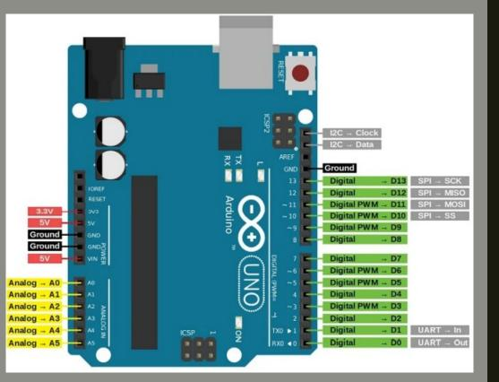
Specifications of *Arduino* UNO Rev3 Microcontroller: *Operating voltage:* +5V (*Recommended*),
